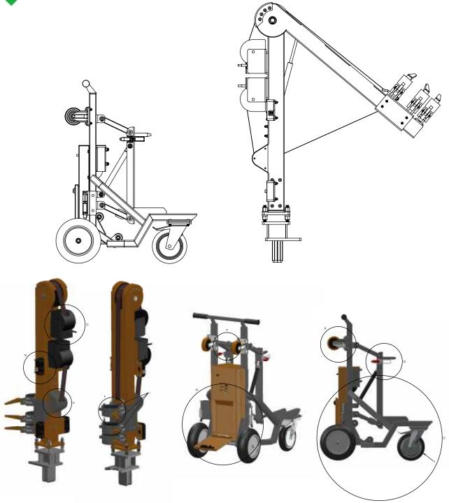
The Patented RS Post Installer is a lifting device designed to be operated during the installation of traffic signal, street lighting and other highway columns which are installed in the NAL Retention Socket System. The design and function of the RS Post Installer facilitates ground level installation and maintenance of the columns and their associated furniture.
