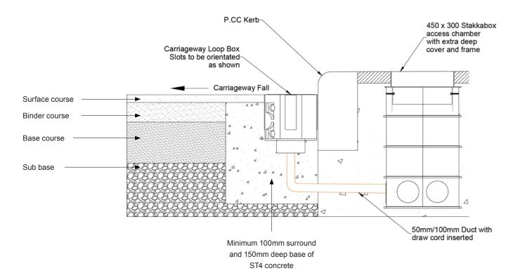
Installation of Loop Box offset from kerb
