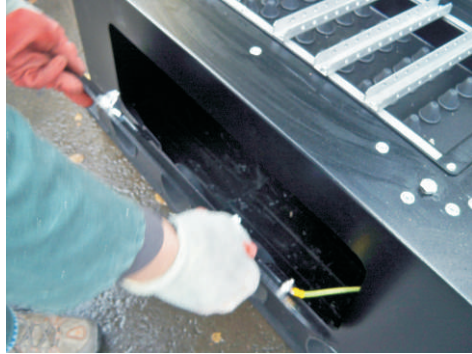
Remove front access door
