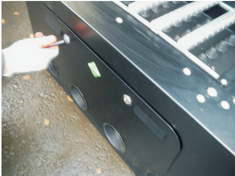
Undo locks on front access door
