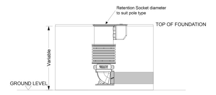
Please see individual Retention Socket drawings for dimensions and individual specifications. Please refer to the NAL installation guide for correct installation and foundation details.
