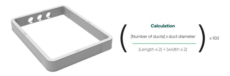
If the ducts amount to more than 30% of a ring section, an **undrilled ring** must be included above it.
