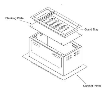
The NAL Controller Base comprises of four components:
